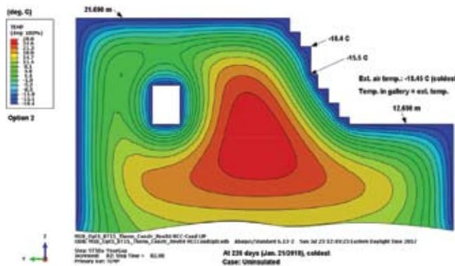
Fig. 7 : Temperature distribution at the coldest winter day (21 Jan 2018) without thermal protection
