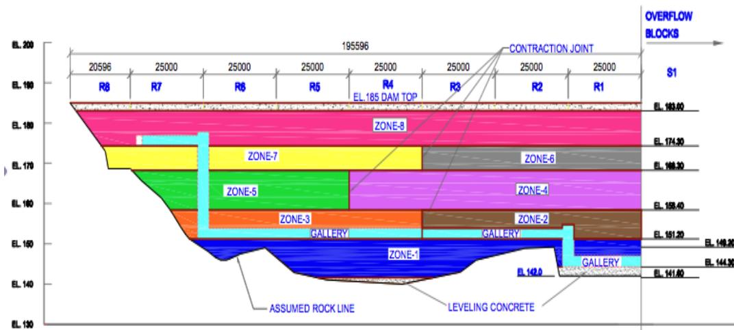
Fig. 2 : Zoning of RCC dam construction
