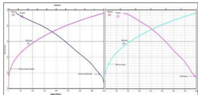
**Fig. 9 :** Elevation area capacity curve for 2005 & 2008 (Left & Right figures)
