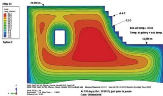
Fig. 6 : Temperature distribution just prior to winter pause (31 Oct 2017).
