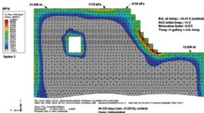
Fig. 11 : Principal stress at coldest external air temperature with no insulation cover.
