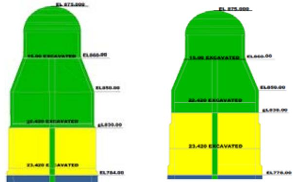
Fig. 14 : Excavated Portion of Both shaft with chamber
