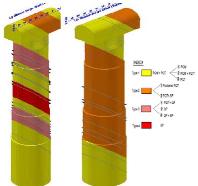
Fig. 5 : 3D Geological model of surge shafts
