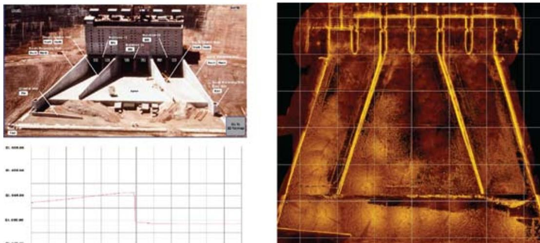
Fig. 14 : Interactive graphic of spillway inspection showing master page derived from construction photo (top l) linked to scan renderings by location
