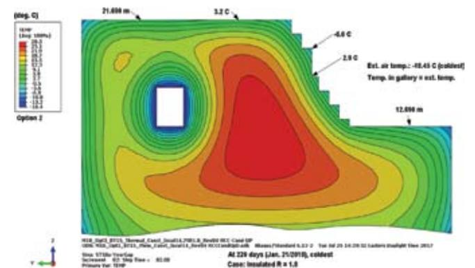
Fig. 13 : Temperature distribution at the coldest external air temperature with insulation covers R1.8
