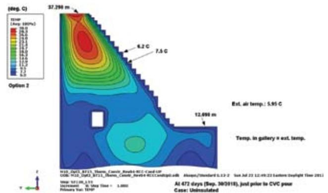
Fig. 9 : Temperature distribution at the completion of the RCC (30 Sep 2018) without protection.
