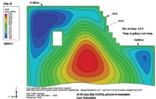
Fig. 8 : Temperature distribution after winter pause (15 May 2018) without protection.
