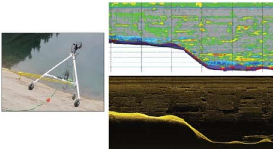
**Fig. 4** : Sonar inspection of dam face. Tripod trolley (l) and detail of relief map (tr) with section scan (br) of the same location.
