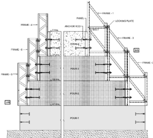
Fig. 6 : Stage - 4 of formwork scheme
