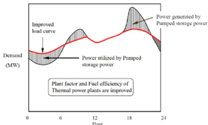
Fig. 1 : Flattening of load curve and improvement of PLF
