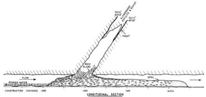
Fig. 6 : Lemonthyme tunnel collapse, determined to be exacerbated by dewatering for inspection
