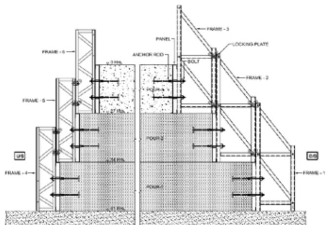
Fig. 5 : Stage - 3 of formwork scheme
