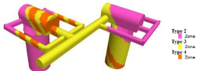
Fig. 2 : Geological model of surge chambers
