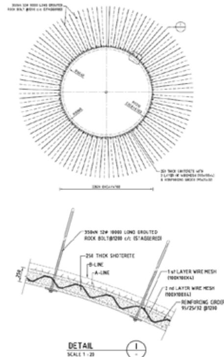
**Fig. 8 :** Typical Support system for Poor rock (PQT+QP, QP, QP+SP)
