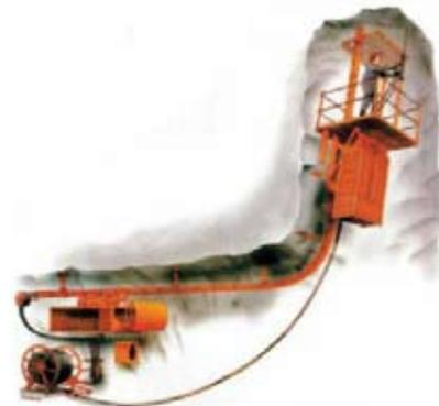
Fig. 11 : Pilot shaft by Raise climber
