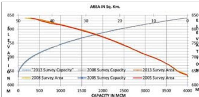
**Fig. 3 :** Elevation capacity curves 2005, 2008 & 2013 survey
