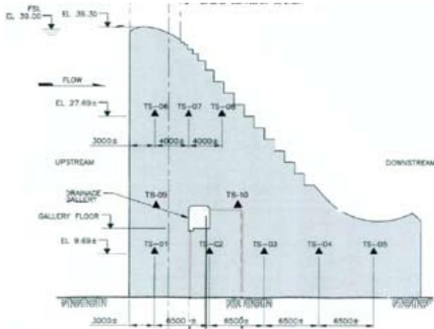
Fig. 18 : Thermistors in the North Dam.
