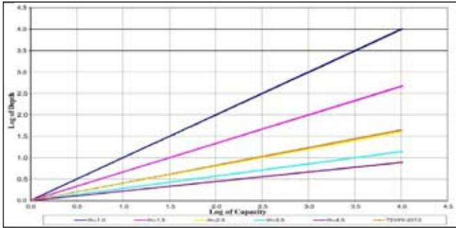
**Figure 5 :** Standard curves for determination of shape of reservoir
