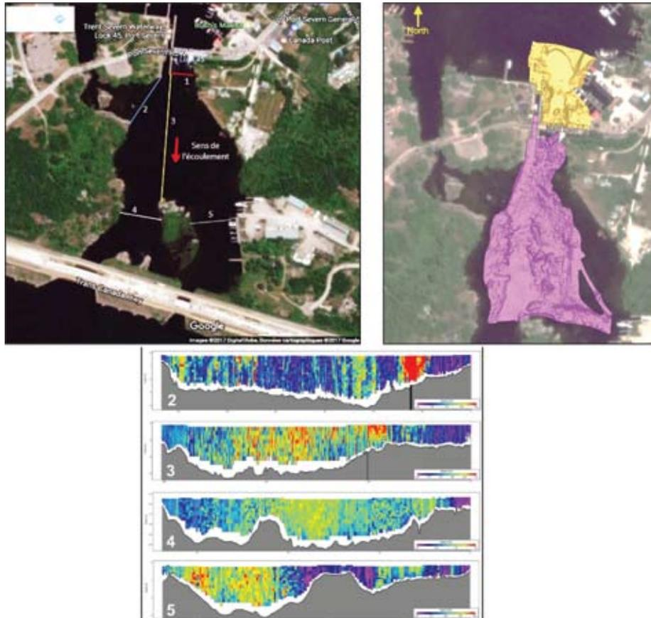
Fig. 7 : Port Severn, Ontario, Hydraulic Velocity Survey Transects. Note the near-shore areas (white) in the heat map in the image on the right, indicating shallow zones that could not be included and therefore omitted from the data set.
