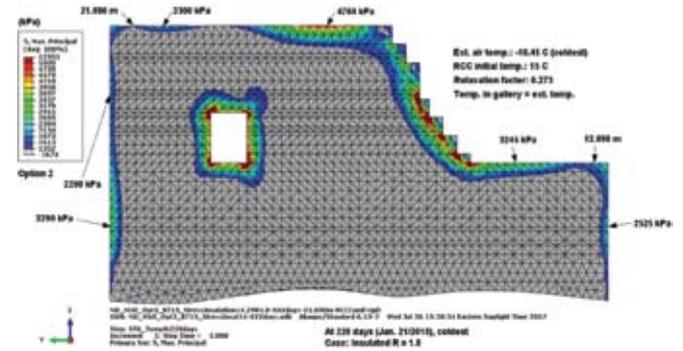
Fig. 12 : Principal stress at coldest external air temperature with insulation covers R1.8
