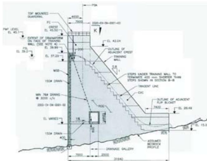
Fig. 2 : General cross-section of North Dam
