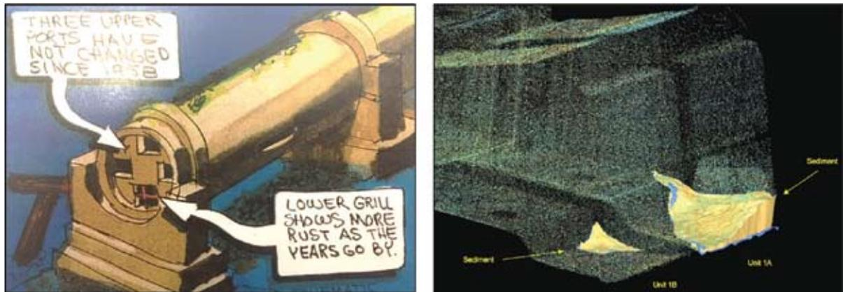
**Fig. 15 :** The old way (anecdotal) inspection drawing of an outfall pipe (l), vs the new way, where metrology derived from the sonar signal allows determination of the actual volume of debris adjacent to an outfall structure (r)
