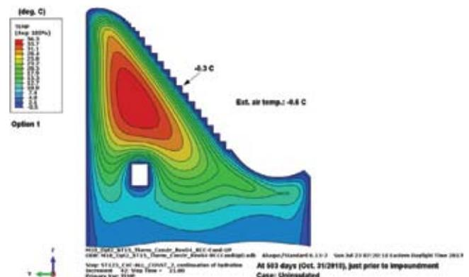
Fig. 10 : Temperature distribution after the completion of CVC ogee (31 Oct 2018) without protection.
