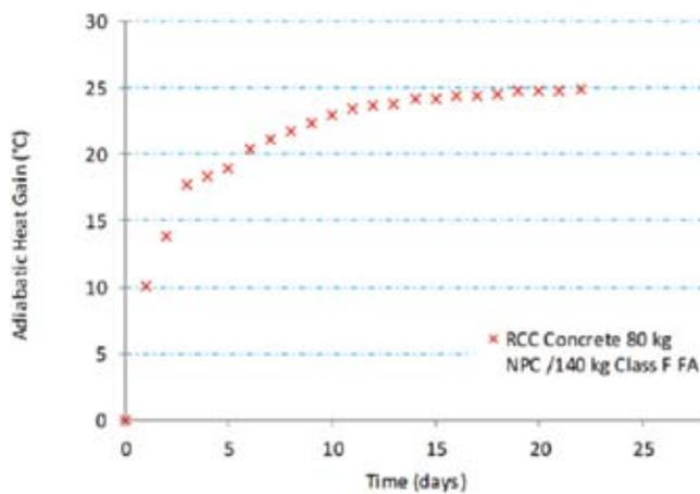
**Fig. 4 :** Adiabatic heat curve for the RCC dam mixture.
