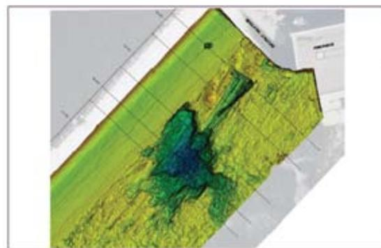
**Fig. 9 :** Multibeam rendering of upstream dam toe and reservoir (r), with sections (l)
