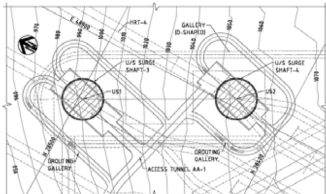
Fig. 1 : Layout of Upstream Surge Shaft
