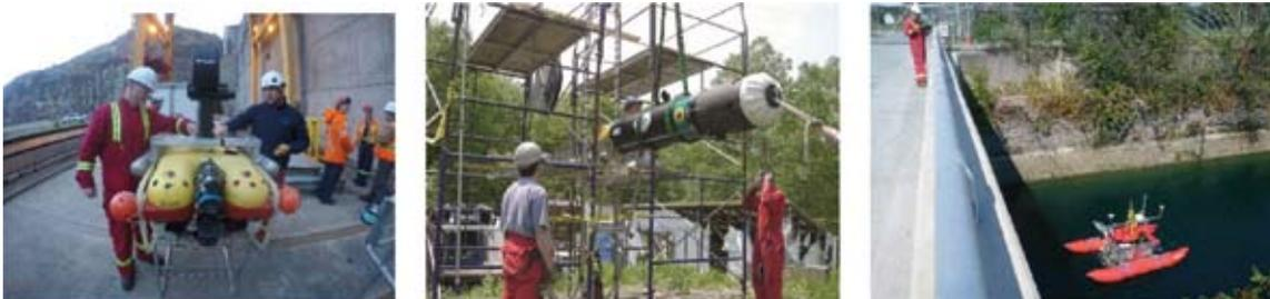
**Fig. 3** : ROV readied for deployment on the Hugh L Keenleyside dam spillway survey (l), AUV launch in NYC's Rondout Pressure Tunnel (c), and ASV deployed at OPG Sir Adam Beck feeder canal (r).
