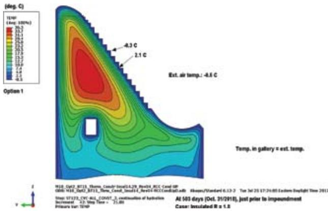
Fig. 14 : Temperature distribution at the completion of CVC ogee (31 Oct 2018) with insulation covers.
