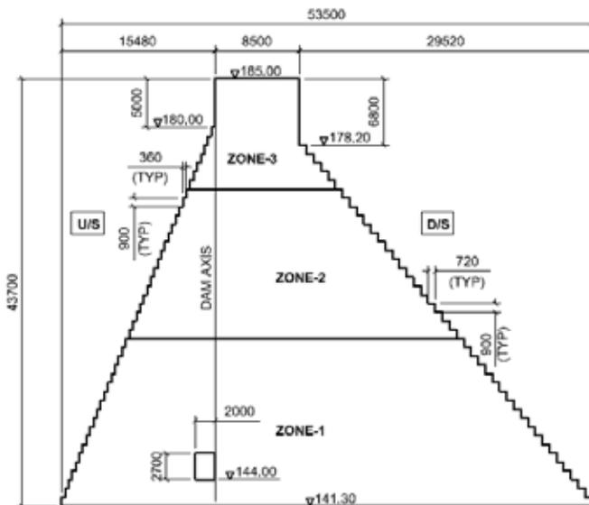
Fig. 1 : Cross-section of RCC dam at TLDP-IV
