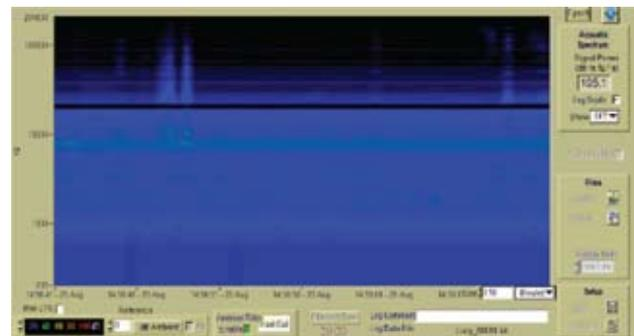
**Fig. 11** : Hydrophone screen capture. Vertical bands indicate noise generated from leaks
