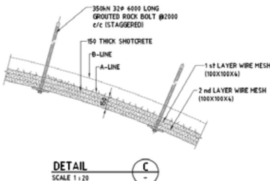
Fig. 10 : Typical support system for Good rock (PQM)
