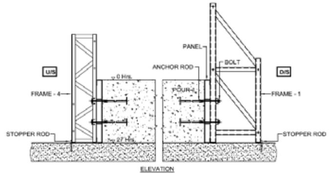
Fig. 3 : Stage - 1 of formwork scheme
